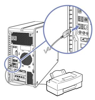
Do not turn on the computer or the printer until all the connections are made.
